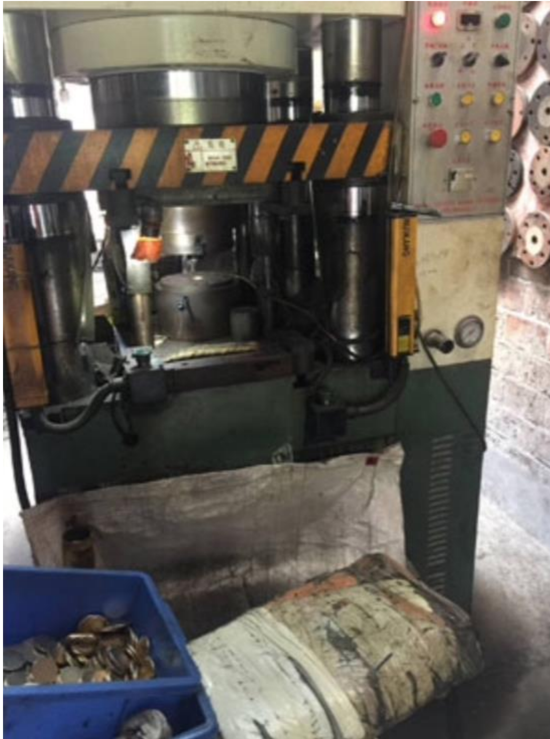
Here is a picture of a Castaing machine used to put edge lettering on the counterfeits.
